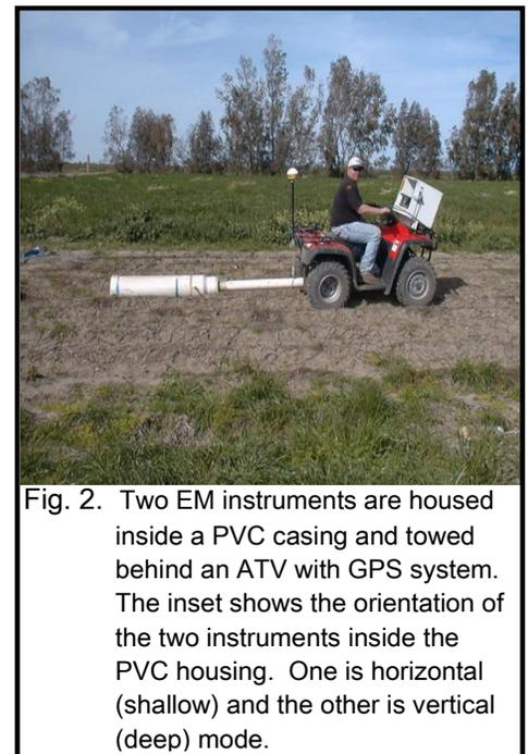
Fig. 2. Two EM instruments are housed inside a PVC casing and towed behind an ATV with GPS system. The inset shows the orientation of the two instruments inside the PVC housing. One is horizontal (shallow) and the other is vertical (deep) mode.
