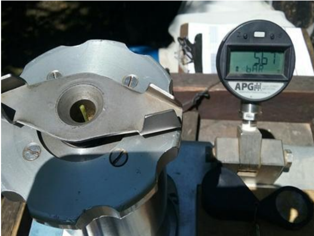
Figure 6. Photo of actual SWP measurement in walnut using a pressure chamber with digital gauge. Plant water status of this walnut tree was -5.67 bars tension. In this example, the length of stem protruding out of the chamber is about \frac{1}{2} inch to help show the end point in this picture. Ideally, the stem should not exceed \frac{1}{8} to \frac{1}{4} inch. Photo: C. Haynes.
